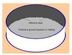
Thoroughly clean the ground again and then lay out the protective matting, with the individual sheets butting up against each other. Cut the protective ground tarpaulin or matting 5 -
