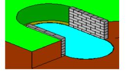
Using a suitable adhesive attach 20 mm-thick Styrodur panels or other insulating panels which are suitable for use in soil to the internal sides of the retaining walls, leaving approx. 25 mm free for the wall tracks above the baseplate.
