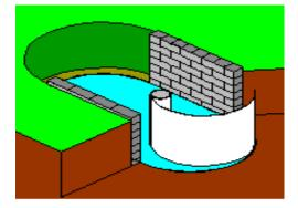
**Caution:** The pre-punched skimmer hole is located approximately 200 cm away from the outer wall end. Make sure when locating the steel wall in the wall tracks that the skimmer hole is also located in the correct required place. In the case of swimming pools with 2 steel walls the skimmer hole is located in Wall 1.
