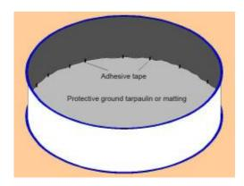
Thoroughly clean the ground again and lay out the protective matting, overlapping the individual sheets by approx. 5-10 cm. Cut the protective ground tarpaulin or matting 5-10 cm larger than the pool outline and tape the resulting overlap firmly to the steel wall. Pull the edges over the wall tracks. To do this, use PVC-compatible adhesive tape (e.g. parcel tape). Pull the protective ground tarpaulin or matting tight to straighten out any creases.
