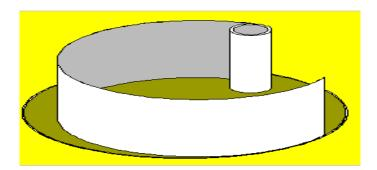
Caution: The pre-punched skimmer hole is located approx. 200 cm away from the outer wall end. Make sure when locating the steel wall in the wall tracks that the skimmer hole is also located in the correct required place. In the case of swimming pools with 2 steel walls the skimmer hole is located in Wall 1.
